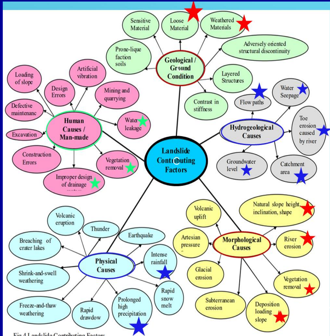
Fig.4 Landslide Contributing Factors
